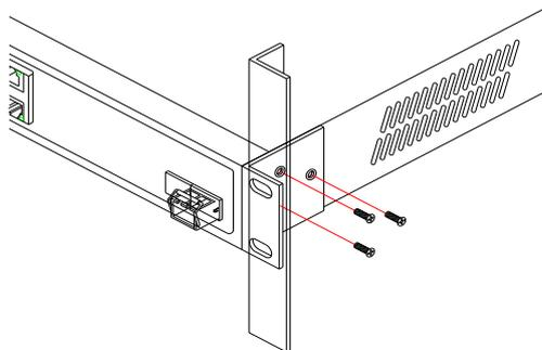
2. Mount the device in the rack using four rack-mounting screws (not provided). Be sure to secure the lower rack-mounting screws first to prevent the brackets from being bent by the weight of the switch.
