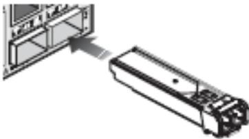
Inserting a SFP Module into a slot
