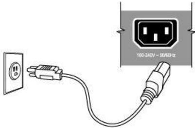
Inserting the power cord to switch and AC power socket
