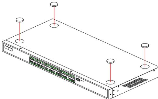
2. Set the device on a flat surface near an AC power source, making sure there are at least two inches of space on all sides for proper air flow.
