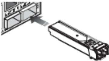
Inserting a SFP Module into a slot
