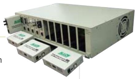
*DCR12 Chassis – front view with Converter Modules*
