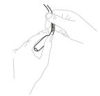
To avoid low or distorted sound, and to provide clear and crisp telephone calls, the microphone should be positioned within 0.5 inches of your mouth. The microphone boom arm will move in a variety of directions to ensure the best fit.
