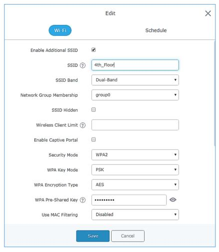
Figure 30: Additional SSID
