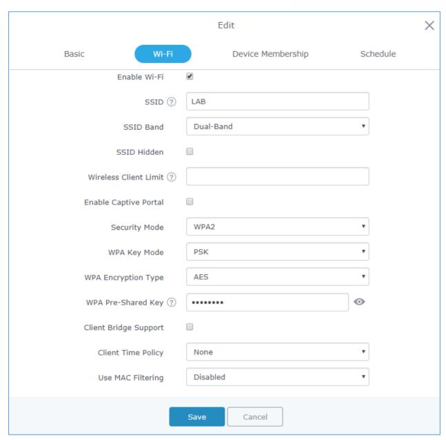
Figure 33: Create an SSID
