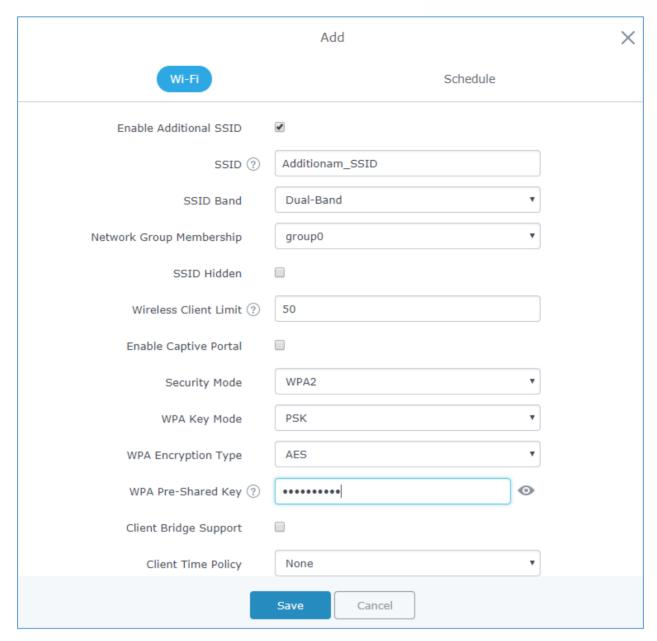
Figure 34: Additional SSID
