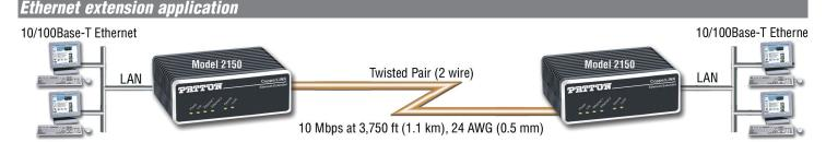
These multi-rate Ethernet Extenders are ideal for bridging Ethernet spans inside buildings that are beyond the 328-foot (100-meter) distance limit of Ethernet.
