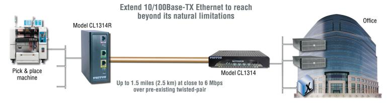
Model CL1314R ruggedized Ethernet Extenders are ideal for delivering Ethernet links to remote buildings that are beyond the 328-foot (100-meter) distance limit of Ethernet. The 5.7 Mbps throughput eliminates bandwidth concerns previously experienced with other copper wired transmission technologies.
