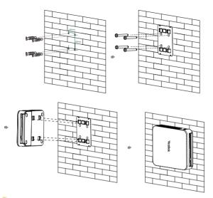
Before mounting the bracket, you need to confirm the direction of the MCore installation. Once the bracket is mounted, the installation direction of the MCore cannot be changed.
