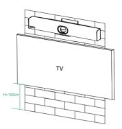
Mount the UVC40 below the TV when the mounting height of the TV is higher than 120cm.
