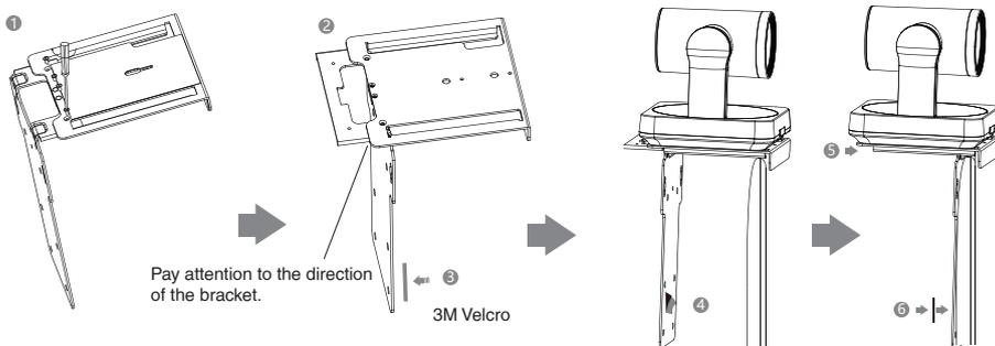
Choose the following installation method when the thickness of the TV is between 50mm and 150mm.
