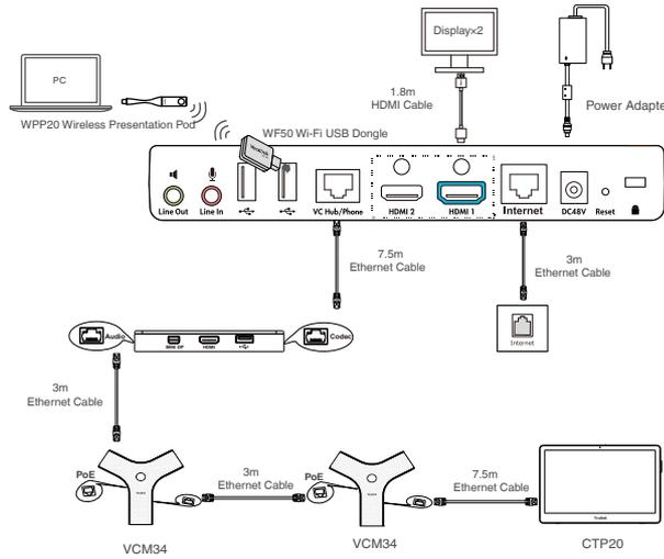
The system should be used with Yealink original power adapter (48V/0.7A) only. The use of the third-party power adapter may cause the damage to the system. The cable should be replaced at once if its skin is broken.
