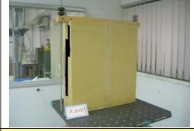
Mechanical shock test: X axis
