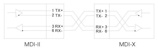
Fig. 5 Straight Through Cable connection
