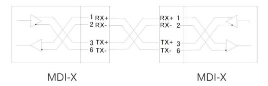
Fig. 6 Cross-Over Cable connection
