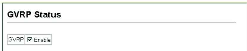
Figure 3-75 Globally Enabling GVRP
