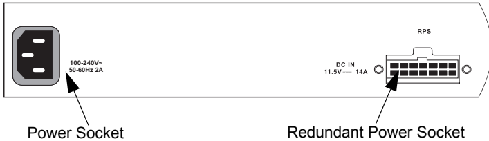
Figure 1-4 Power Supply Receptacle
