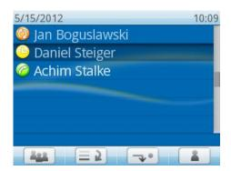
The menus for presence, contact list, etc. will dynamically switch their context according to the current active identity selected (highlighted) via the Navigation button on the device.
