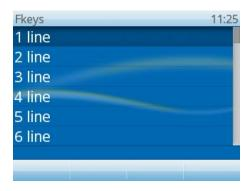
Select the key to which the Boss/Admin should be assigned to (the text behind the number shows the current configuration).
