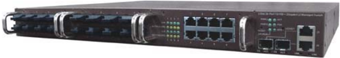
Fig. 1-1: Front View of the MS888G2 Switch with modules
