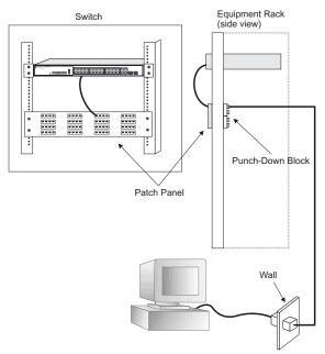
Figure 4-2 Network Wiring Connections
