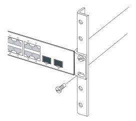
Figure 3-3 Installing the Switch in a Rack
