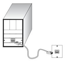
Figure 4-1 Making Twisted-Pair Connections
