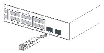
Figure 3-5 Inserting an SFP Transceiver into a Slot
