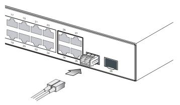
Figure 4-3 Making Connections to SFP Transceivers
