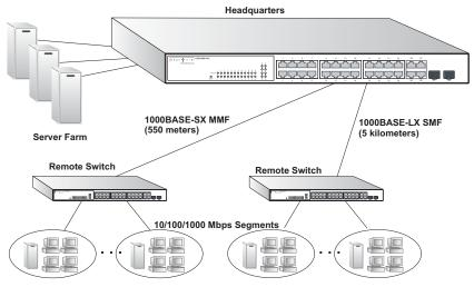
Figure 2-4 Remote Connections with Fiber Cable
