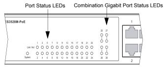
Figure 1-2 Port Status LEDs
