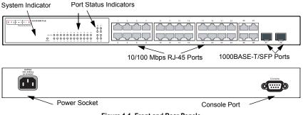
Figure 1-1 Front and Rear Panels
