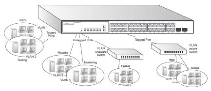
Figure 2-5 Making VLAN Connections
