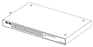
Figure 3-4 Attaching the Adhesive Feet
