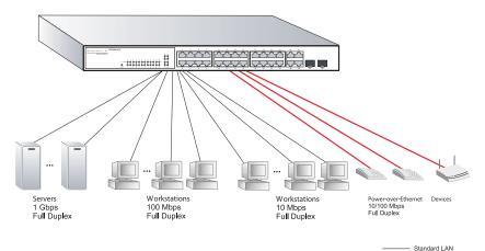
Figure 2-2 Collapsed Backbone
