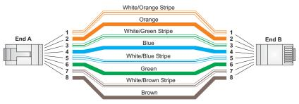
Figure B-2 Straight-through Wiring
