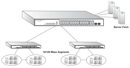
Figure 2-3 Network Aggregation Plan
