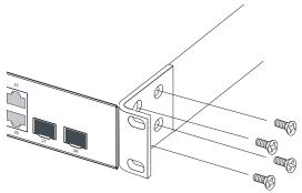
Figure 3-2 Attaching Brackets for Rack Mounting
