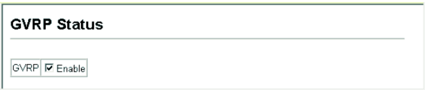
Figure 23-1 Globally Enabling GVRP
