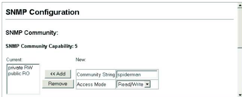
Figure 3-24 Configuring SNMP Community Strings
