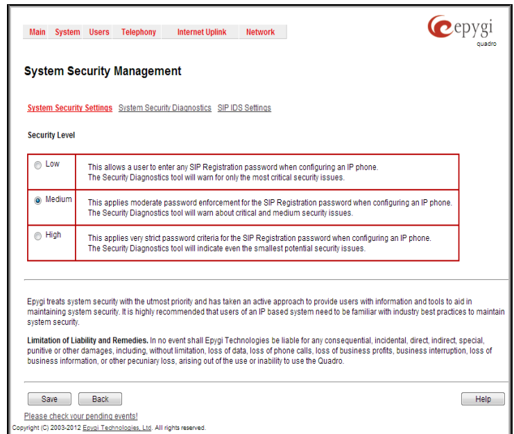
Fig. II-11: Quadro FXO 4 System Security Management page
