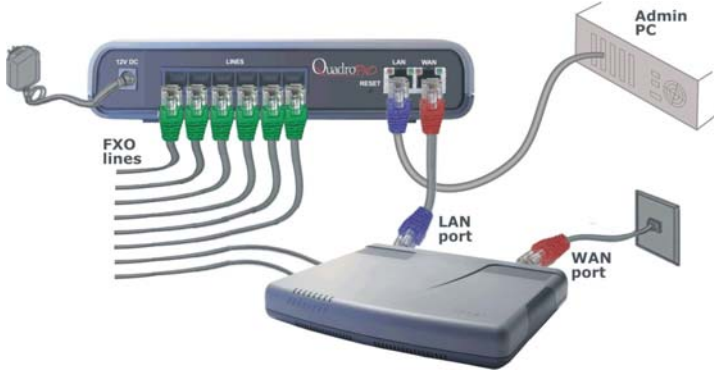
Fig. I-29: Installation of QuadroFXO as a LINE expansion for a Quadro IP PBX
