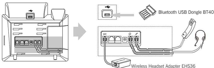
Note: The headset, Bluetooth USB dongle BT40 or wireless headset adapter EHS36 should be purchased separately. The EXT port can also be used to connect the expansion module EXP40. For more information on how to use the EHS36, EXP40 and BT40, refer to Yealink EHS36 User Guide, Yealink SIP-T46G Microsoft Skype for Business Edition User Guide and Yealink Bluetooth USB Dongle BT40 User Guide.
