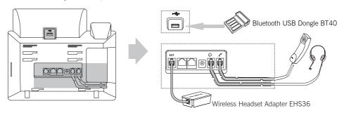
Note: The headset, Bluetooth USB dongle BT40 or wireless headset adapter EHS36 should be purchased separately. The EXT port can also be used to connect the expansion module EXP40. For more information on how to use the EHS36, EXP40 and BT40, refer to Yealink EHS36 User Guide, Yealink SIP-T48G Microsoft Skype for Business Edition User Guide and Yealink Bluetooth USB Dongle BT40 User Guide.
