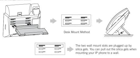
Note: For more information on how to mount the IP phone to a wall, refer to Yealink Wall Mount Quick Installation Guide for Yealink IP Phones.
