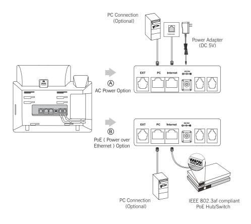
Note: The IP phone should be used with Yealink original power adapter (5V/2A) only. The use of the third-party power adapter may cause the damage to the phone.
